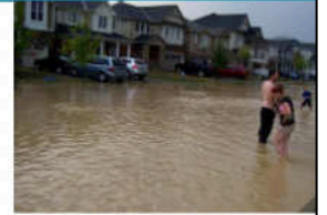
Basement flooding can occur even where well-defined major drainage systems are present, due to excess water entering sanitary sewers. Regional basement flooding occurred during this storm in Binbrook, where ~250 mm of rain fell in 3 hrs. (Photo: Weather Network).
