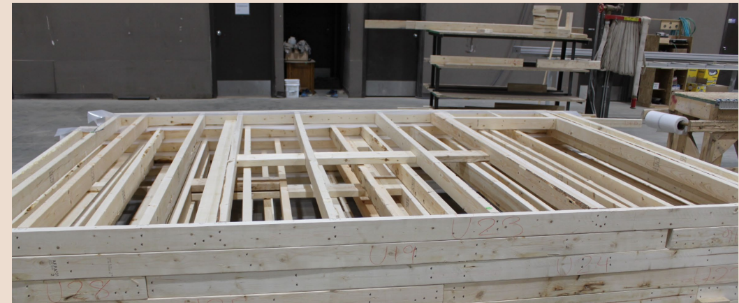
Factory built wall panels
