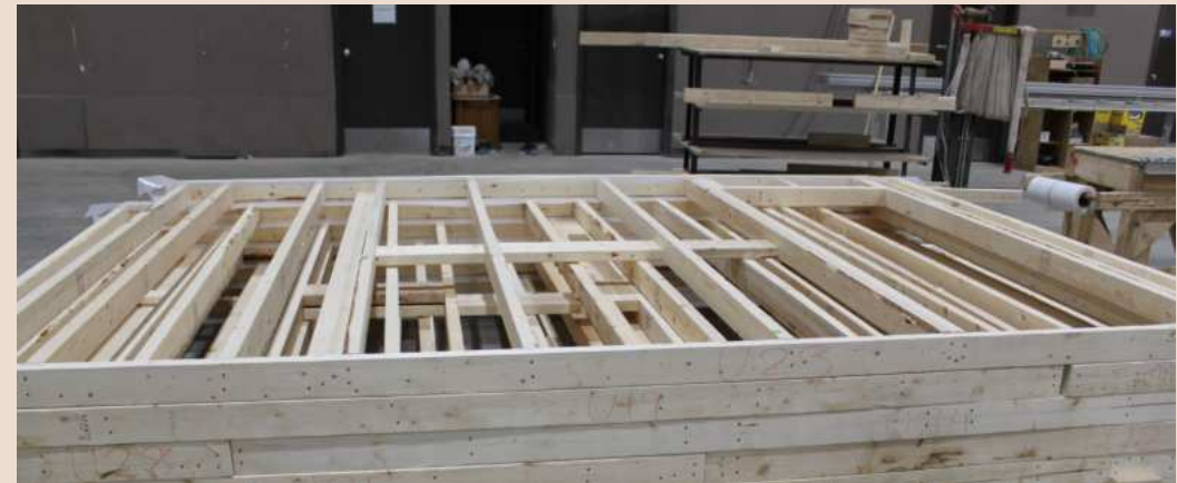
Factory built wall panels
